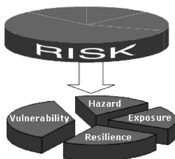
Figure 23.4 Risk seen as a function of hazard, vulnerability, exposure and resilience, while the mathematical relationship between the variables is unknown.
