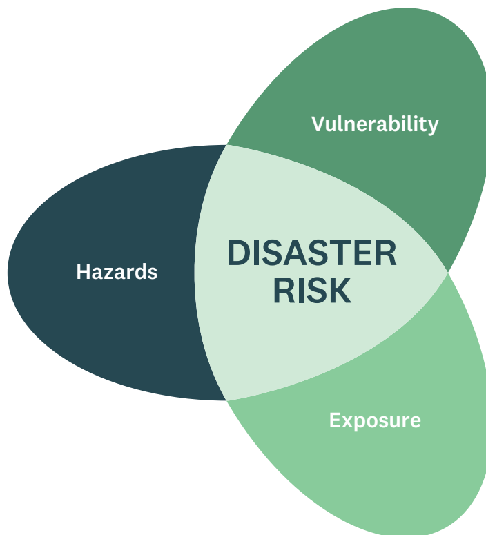
Figure 3 - Risk propeller showing risk being composed of hazard, exposure and vulnerability. Adapted from IPCC, 2014
