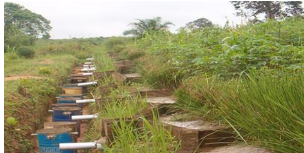
Sedimentation drums installed in the ground in a trench dug at the lower end (down slope) of the erosion plot, with vetiver buffer serving as erosion control measure.
