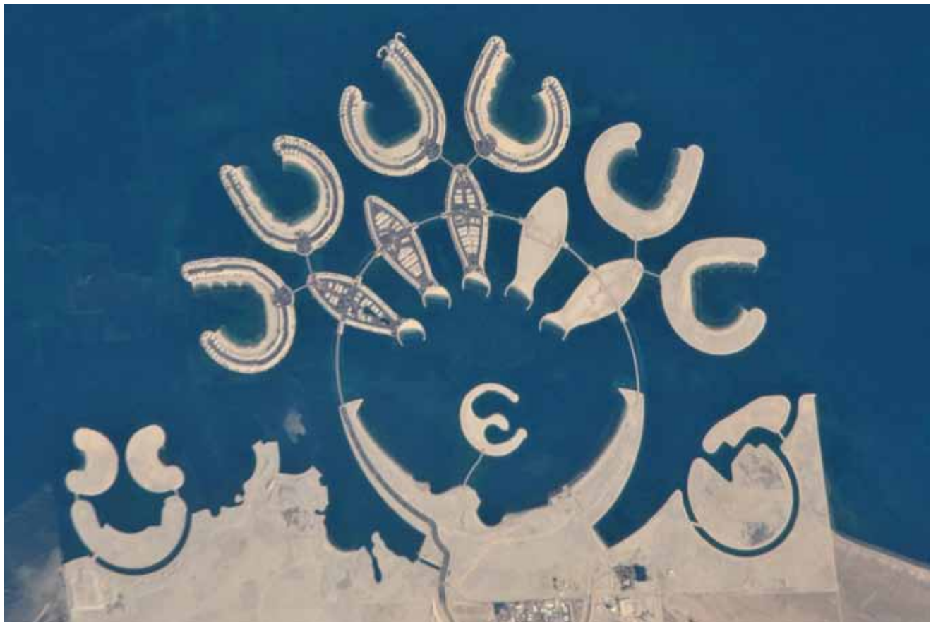
Figure 3. Durrat Al Bahrain, still under construction in Bahrain, will be a new (near shore) mega-island city with 15 interconnected islands that will cover 20 km 2 . Credit: NASA Earth Observatory
