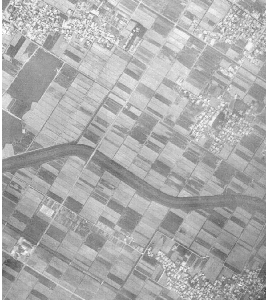
Figure 4.11 A recent rural landscape after land consolidation, with separate ditches for drainage and water supply (common since the 1970s)
