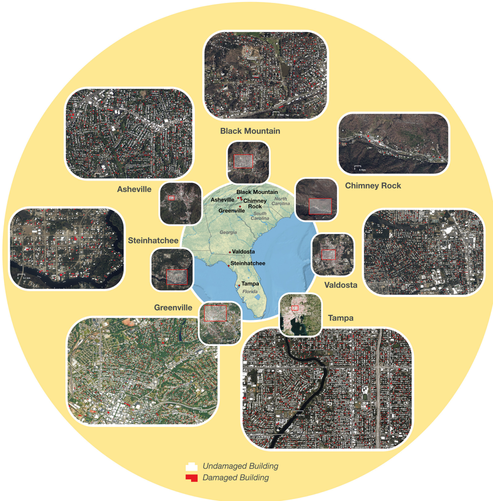
Figure 1. Building damage map. Damage probability for each building is calculated by applying a Bayesian image classification framework 4,5 to the interferometric coherence map of a SAR interferogram covering the hurricane event. Buildings with a damage probability exceeding 99% are highlighted in red for clear identification.
