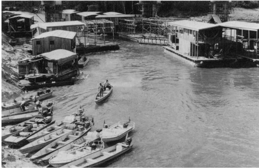
Figure 6.8 The frenzied scramble to build suction dredges ( dragas ) for operation on the Madeira River, whose alluvial channel deposits have been counted among the world's richest sources of riverine placer gold. The dragas incorporate a platform supported by two iron cylinders some 14 m in length, and a structure that houses the machinery and includes the operators' living quarters (a smaller and more rudimentary version are the balsas ). The river gravels are worked by a powerful cutterhead at the extremity of a lance, while a diesel-driven pump draws in the slurry. After the gold particles are trapped and concentrated in a sluice, liquid mercury is used in amalgamation. Although every dredge now is theoretically required to employ a retort to recover the mercury for reuse, the amalgam is often heated over an open flame (Veiga, 1993). In this case, the vaporized mercury is eventually precipitated, polluting soils and waters. A paper accepted for publication in 1986 refers to some 100 dragas in operation along a 180-km stretch of the Madeira River upstream of Porto Velho (Bastos, 1988). Their number was reported to have reached 5,000 in 1989 (Hilde, 1989) and 10,000 in 1990 (Dias, 1993); however, a possible source of uncertainty in the count is the inclusion of balsas in some reports. After this peak, the number of dragas fell off sharply, and many, having been built at a cost of several kilograms of gold each, were abandoned on the riverbanks. The drop is attributed by some to a partial exhaustion of recoverable gold (Veiga, 1993) – at least in terms of the low efficiency of the dragas . (Photographed 6 June 1989.)
