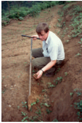
Figure 4.14b: Using a Soil Auger
