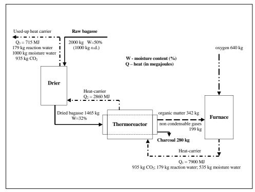
Figure 9. Material and energy flows using LSIWC charcoal energetically self - sufficient production technology as case study [25].
