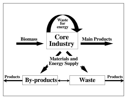
Figure 8. Self-supporting with materials and energy sugar cane mill and complementary industries cluster [23]. The main products from the core industry are sugar and/or alcohol; by-products are molasses; waste is sugar cane bagasse.
