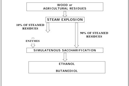
Figure 5. A simplified process of biomass conversion to ethanol or butanediol using steam explosion and SSF according to E.K.C.Yu and J.N.Saddler
