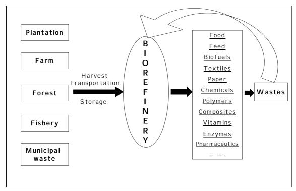
Figure 1. Closed loop: biomass - biorefinery - value added products - disposed waste - biorefinery.
