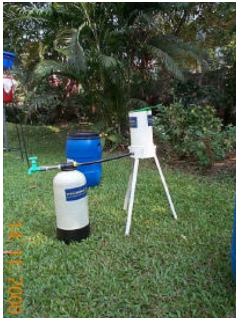
Figure 6: Tetrahedron Ion Exchange Resin Filter
