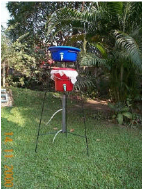
Figure 2: BUET activated alumina filter
