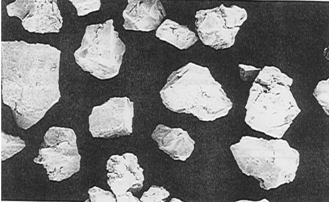
Figure 2 : AdsorpAs® - synthetically manufactured Iron Hydroxide having a porosity of about 75% and specific surface of 250 – 300 m 2 /g.
