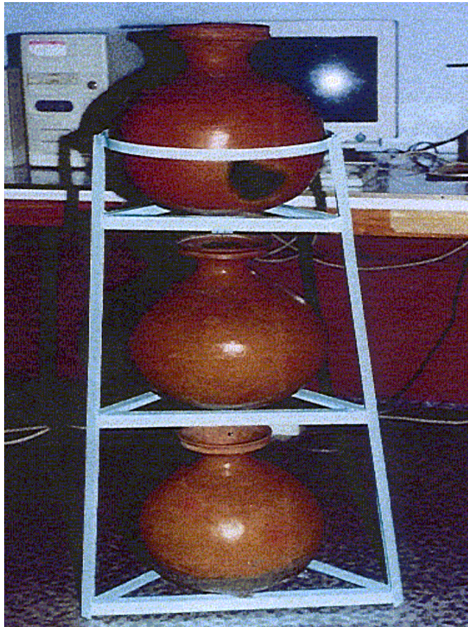
Figure 1: Picture of a 3-Kolshi-filtration setup. This particular setup was used to filter 6000 L of arsenic contaminated groundwater. The computerized electrochemical analyzer for the measurement of arsenic is shown in the background,
