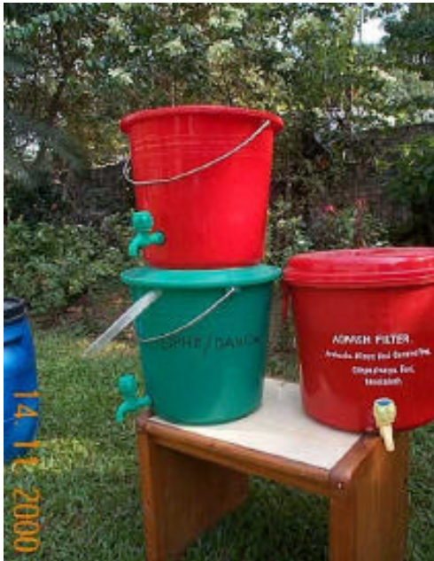
Figure 4 : DPHE-Danida Bucket Treatment Unit (BTU)
