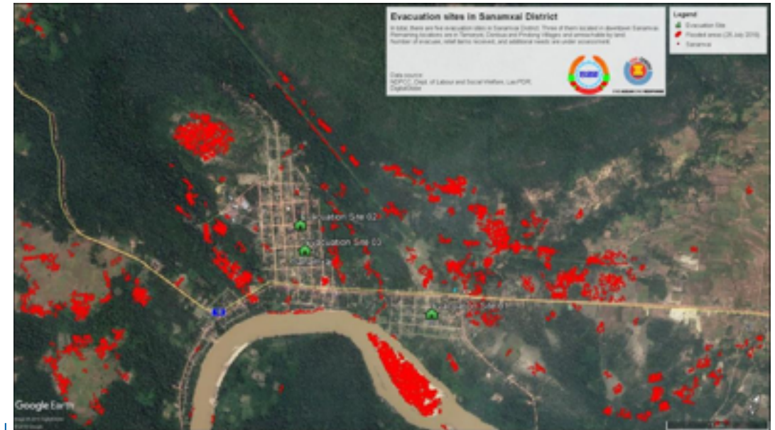
Figure 10.8 Use of Satellite-based observation 2: Overlay of Inundation Areas for determining location of Mobile Storage Unit
