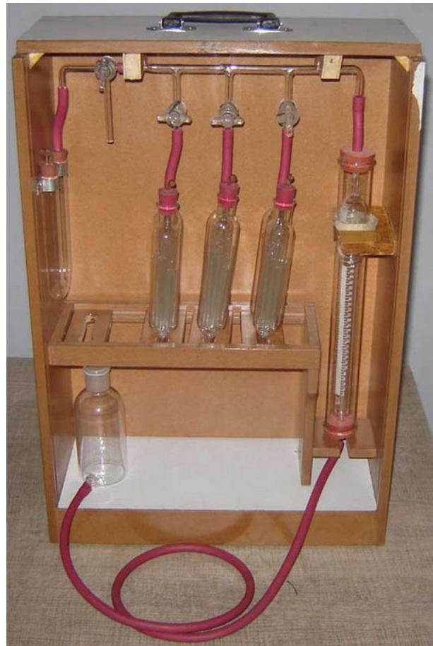
FIGURE 11: Image of an Orsat apparatus used in measuring relative CO 2 abundance in soil. (courtesy of EEE Ltd, 2016)
