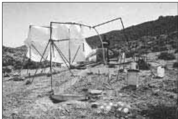
Photo 5.3: Rainfall simulation tests at the Amrich jessr impluvium
