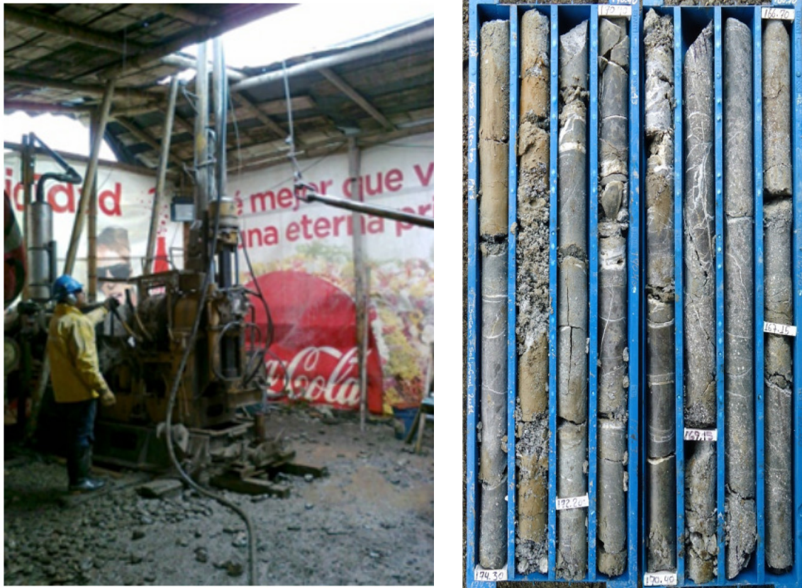
FIGURE 3: Left, rig used for TGW 1; Right, cores obtained, mainly andesites with fracture zones and propilitic alteration crossed by calcite veins
