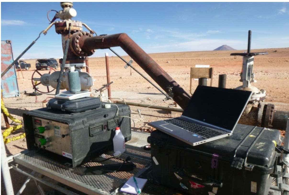
FIGURE 1: Installation of MicroMod Tracer Injection Unit (TFT method) during well testing of SM – 03 in February 2013
