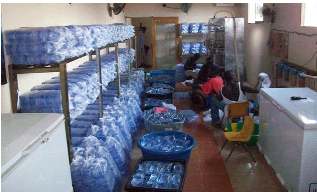
Figure 4: A simple production line for sachet bag water.
