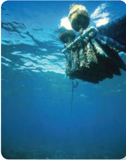
Figure 29. Examples of experimental collectors used in spiny lobster connectivity studies to capture postlarvae as they recruit to back-reef nursery habitats. The above photo is a Witham-type collector used to collect Caribbean spiny lobster. The below photo shows an experimental apparatus designed to attract Caribbean lobster postlarvae and then provide housing for them in crevice structures as they grow larger. Photo: Mark Butler (above); Unknown (below)
