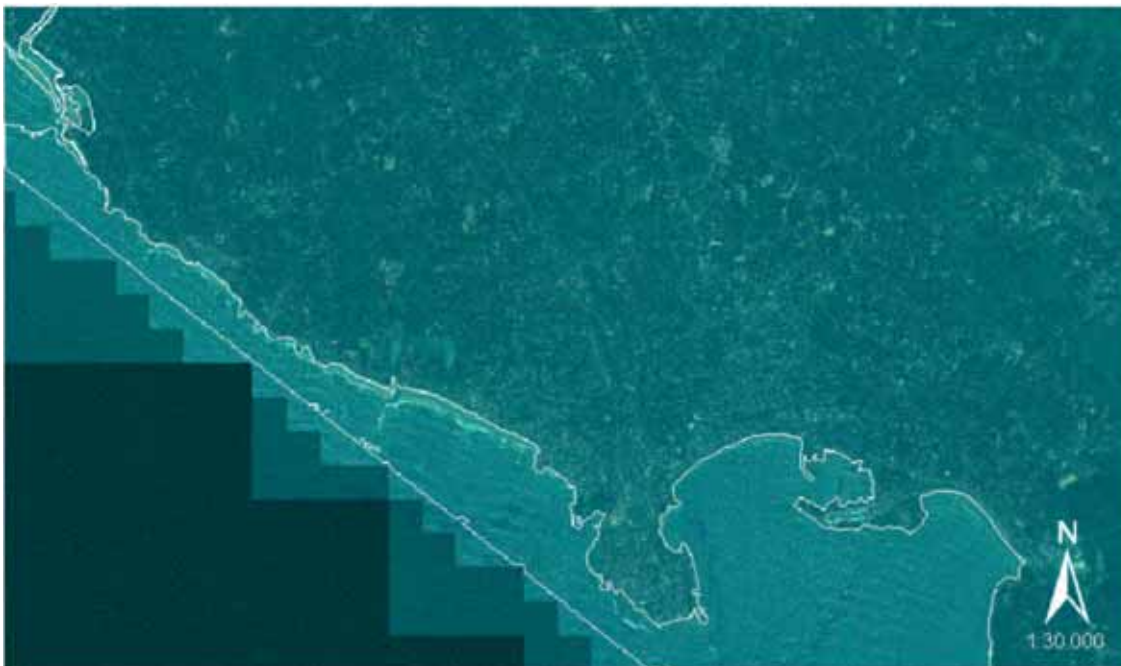
Figure 5: Automatically derived shore line based on multispectral properties
